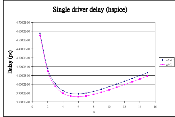
Fig. 3. Effect of ignoring wire resistance on delay
